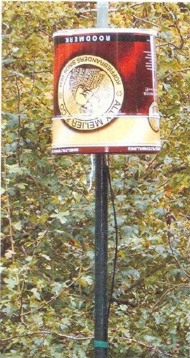
*Photo 6 - Passive E-field antenna.*
