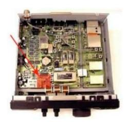
•Locate resistor R1102 (1.5k ohms) as pointed to by the red arrow in the picture below. Using a magnifier you will note the resistor has the marking '152' that stands for 1500 ohms. You can check this via multimeter. Note that pins 2 and 3 of the mixer (MC1496; see green underline) attach directly to R1102 as per the schematic above.
